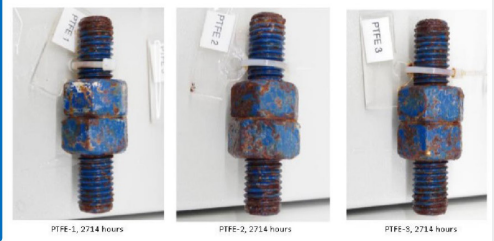
Xylan @ 2,714 hours ASTM B117 Salt Spray
