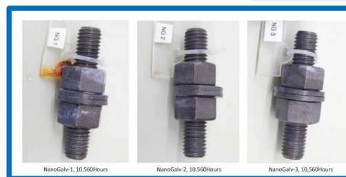
NanoGalv® @ 10,560 hours ASTM B117 Salt Spray
